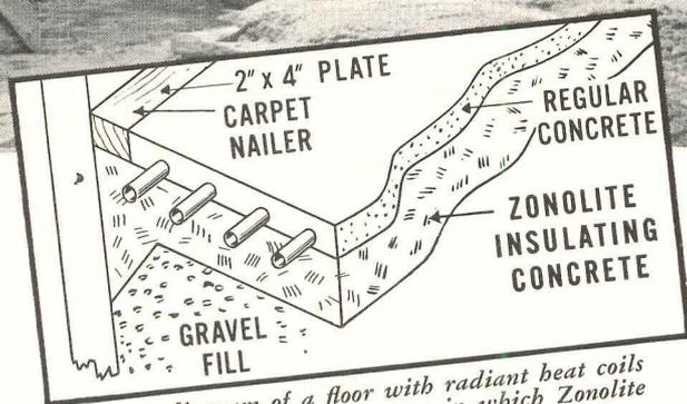
*This diagram of a floor with radiant heat coils shows one of the many ways in which Zonolite Vermiculite Concrete can be used efficiently.*
