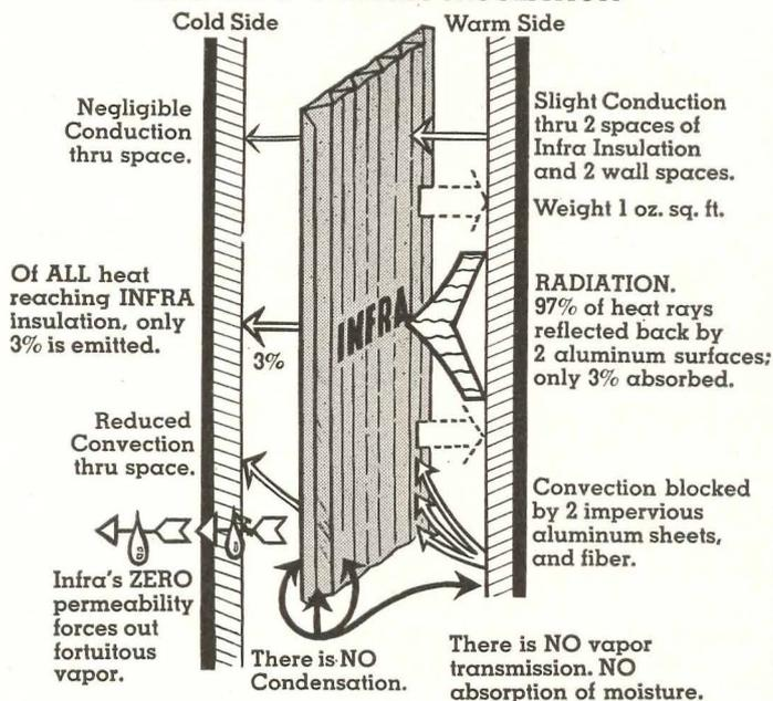
MULTIPLE ACCORDION ALUMINUM and TRIANGULAR REFLECTIVE AIR CELLS
