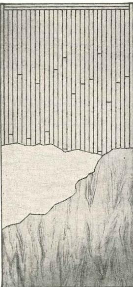
Unusual versatility makes this new addition to the Weldwood line a favorite with architects everywhere. Because of its solid lumber staved core construction, the door can be hung from either side. Hardware is easily installed in any standard or custom position. Lights and louvers may be cut on the job.
