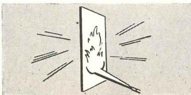
**Fire Resistance**—One reason why Roddiscraft Solid-Core Flush Veneered Doors are ideal for hospitals is their exceptional resistance to fire. This fact has been established by independent laboratories, where standard Roddiscraft doors exceeded the 40-minute fire test.
