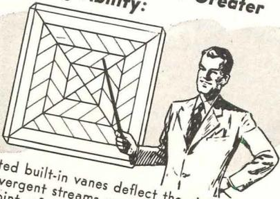
Patented built-in vanes deflect the air in numerous divergent streams resulting in turbulence at the point of contact with the aspirated air. Result: Rapid mixing, diffusion and temperature equalization.
