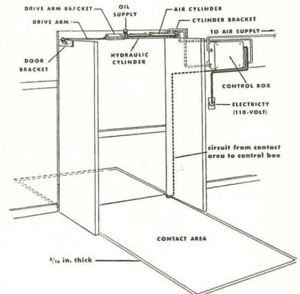
Door control uses no motors or gears
