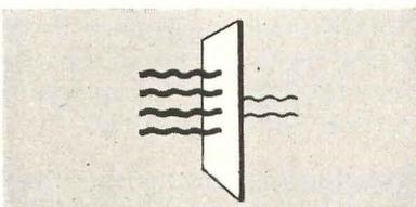
**Sound Resistance**—The high resistance of Roddiscraft solid-core construction to the passage of sound has been established by independently conducted laboratory tests. The standard 1 3/4" Roddiscraft Solid-Core Flush Veneered Door develops an average sound transmission loss of 30.9 decibels.
