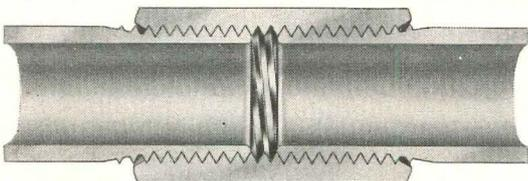
**ORDINARY COUPLING**—Raw threads meet raw threads—accelerates rust—weakens joint. Threads exposed in gaps trap wire ends and make the fishing of wires difficult.
