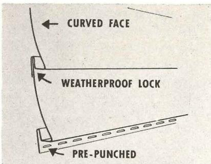
**CURVED SURFACE**, installed under tension, makes rigid, sound-resistant, insulating siding with weatherproof joints, beautiful shadow lines without wrinkles. Easy to apply. Low construction costs!
