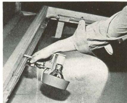
Wiring duct holds fixtures at any point
