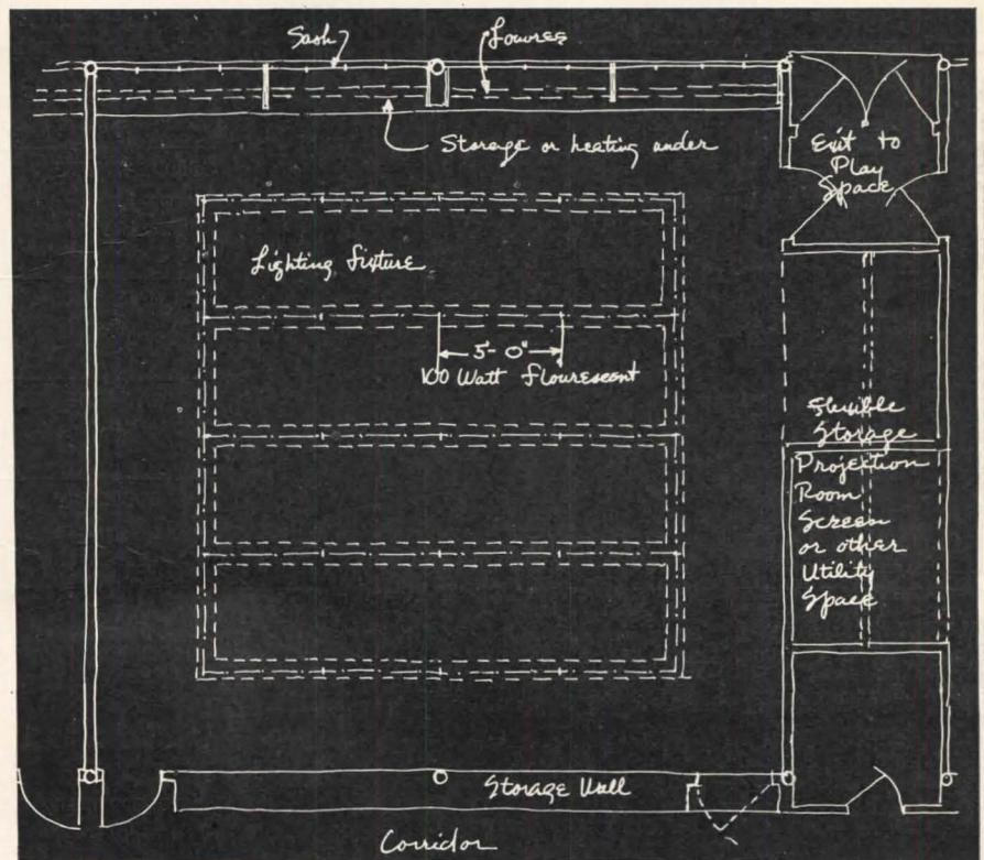
Fixture pattern is seen in plan, above. As drawn, it uses 28 100-watt F lamps, with auxiliaries, the output becomes 117,600 lumens.
