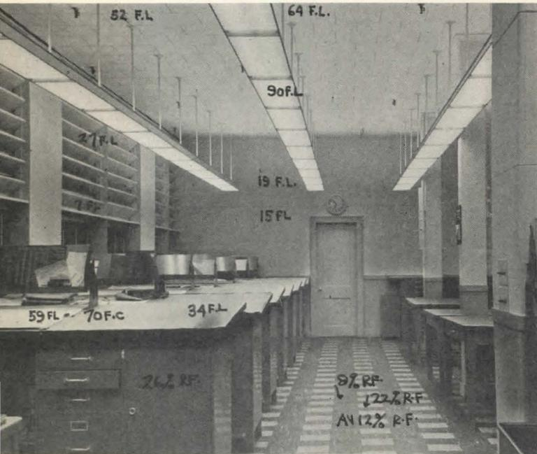
Below, same room by day. Brightest area, the window louvers, is held down close to ratio of 3 with work. Inner wall is in need of supplementary artificial lighting to keep brightness even
