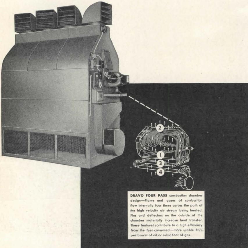
**DRAVO FOUR PASS** combustion chamber design—Flame and gases of combustion flow internally four times across the path of the high velocity air stream being heated. Fins and deflectors on the outside of the chamber materially increase heat transfer. These features contribute to a high efficiency from the fuel consumed—more usable Btu's per barrel of oil or cubic foot of gas.
