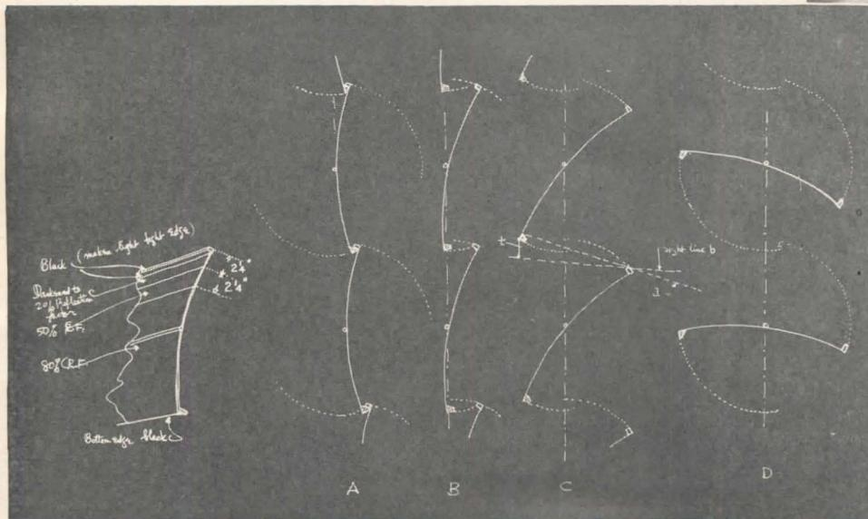
Sight-lines "a" and "b," seen somewhat faintly in the diagram above, correspond to the sight-lines marked the same way on page 116, in the diagram of the room as a whole. It may be seen why a tab or flap (t) is needed to eliminate skyglare entirely when this louver is part-way open. At left are suggestions for graded reflectivity of the louver, to distribute reflections evenly; also, lower reflectivity of upper edge permits wider opening
