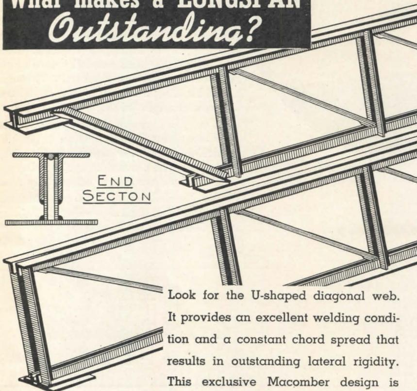
Look for the U-shaped diagonal web. It provides an excellent welding condition and a constant chord spread that results in outstanding lateral rigidity. This exclusive Macomber design is made in underslung or square end types with sloping or parallel chords in lengths up to 70 feet. Here is a completely standardized structural unit, specified from load and span tables for unobstructed floor or roof support. Get our complete design information for your next project.
