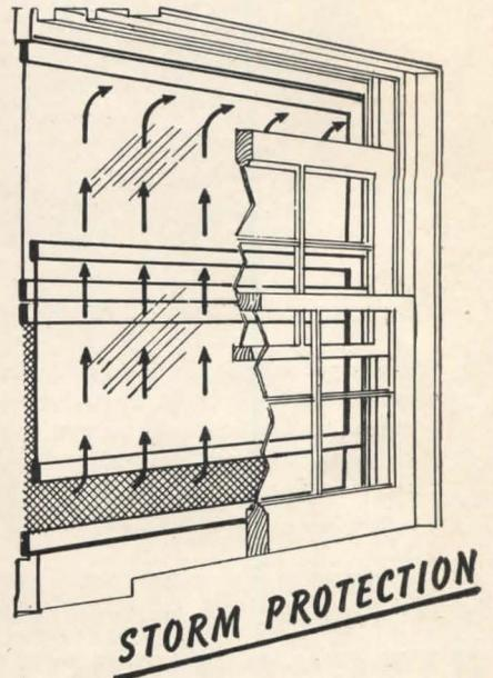
Stormproof, draft-free ventilation winter or summer by raising lower Rusco sash part way, lowering upper inside sash. Air deflects upward into room—permits open window ventilation with complete safety from storm damage or drafts.
