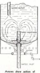
Arrows show action of water when drawn thru TURBO-AQUATHERM scouring bottom of boiler and preventing any accumulation of sediment
