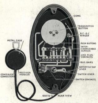
Rear View—Showing Mechanism in Detail
