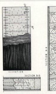
Hyde-Murphy guaranteed "No-Warp" flush doors are made 5 ply, with framed up cores sanded to even thickness on which are applied 1/2" cross banding and standard 1/8" face veneers. All veneers and cross banding are applied under hydraulic pressure of not less than 2,500 lbs. and the finished doors are laid flat under continued pressure and dried for two weeks. They are absolutely guaranteed for one year from delivery date against defects in materials or workmanship.
