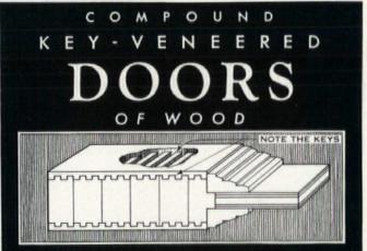
Having more than twice the glueing surface of ordinary construction, key-veneered doors are unequalled in their servicable qualities. Testimony of their desirable characteristics is evidenced by the 30 years or more they have endured in nationally known buildings.<sup>\*</sup> Furnished in any reasonable design or size.
