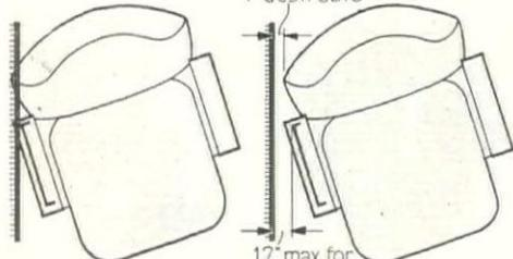
**INCORRECT**—Standard set tight against wall, if at angle, causes seat back to scrape
