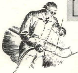
The welds, "W", are smooth inside and flush with the pipe wall on the outside. Each weld is inherently more simple than any other joint can possibly be.
