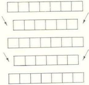
Seats should be aligned at aisles. Banks of staggered seats such as those often used abroad cause jagged aisles with "pockets" which hamper exit of an audience. An additional problem is introduced when finish aisle flooring differs from general seating area flooring or when the aisle is heavily carpeted.
