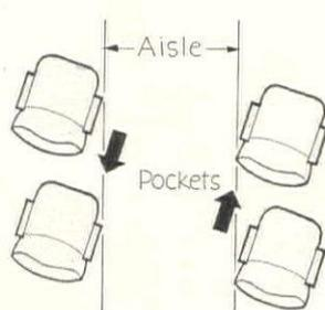
Aisles cutting diagonally across rows produce dangerous "pockets" and waste space
