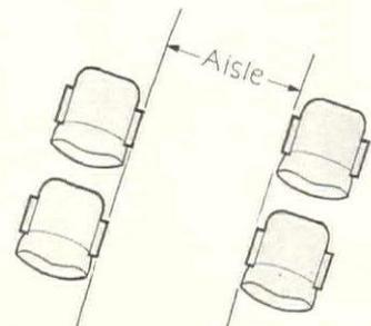
Curved or straight radial aisles reduce number and size of "pockets"
