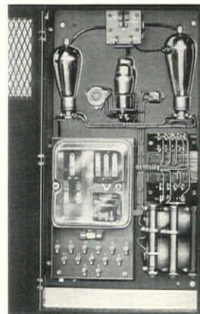
Ward Leonard Electric Co., Mount Vernon, N. Y. has developed two automatic electronic alternator voltage regulators. They have no moving parts. Instead of relying upon mechanical means to close contacts or change pressures an inertialess stream of electrons controls the regulating action. These regulators are controlled rectifiers deriving their power from the a.c. generator and delivering the rectified d.c. current to the shunt field of the exciter in an amount which is a function of
