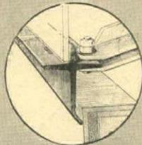
Patented sill member. Drip holes prevent pocketing water when sash is open. Opposite flanges take thrust of operator without strain on glass
