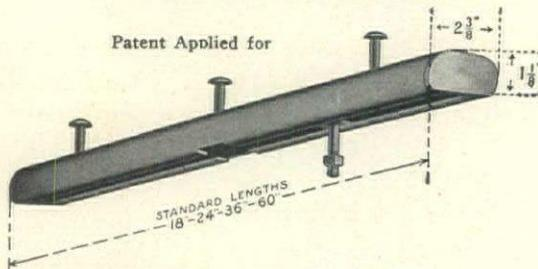
Manufactured from the highest grade of pressed steel and suitable for 5/8" or 3/4" bolts. Only 1 1/8" deep, permitting reinforcing steel to pass over it without reducing the strength of the construction.
