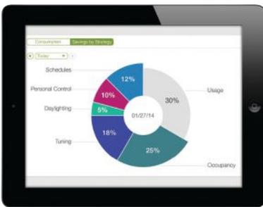
Quantum Vue is an easy-to-use facility management tool you can use on any device. Access building performance and energy data, as well as monitor, control, and optimize a Lutron light and shade control system. Quantum Vue also provides hassle-free scheduling and real-time tuning.
