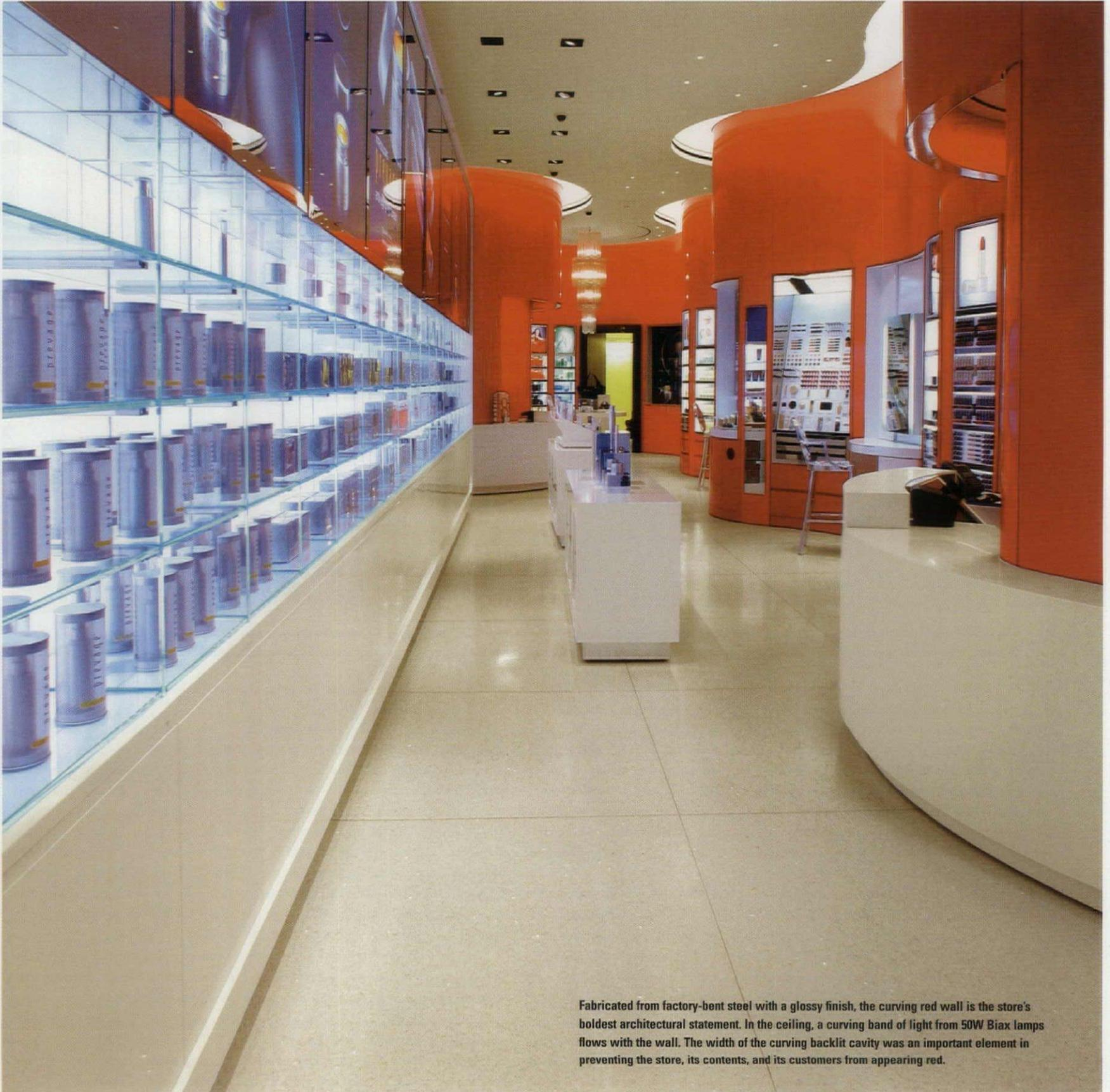
Fabricated from factory-bent steel with a glossy finish, the curving red wall is the store's boldest architectural statement. In the ceiling, a curving band of light from 50W Biax lamps flows with the wall. The width of the curving backlit cavity was an important element in preventing the store, its contents, and its customers from appearing red.
