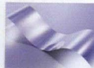
MICRO-MATT™ by ALANOD is specular; it controls light direction, producing up to 20% more light to the task than the same luminaire using a white paint reflector. Yet, MICRO-MATT appears white. Unlike MIRO, white painted reflectors are highly diffused, offering little optical control. They have a polar light distribution unsuitable for vertical illumination. MIRO MICRO-MATT provides the aesthetic appearance of a white surface yet with vastly improved light controllability.
