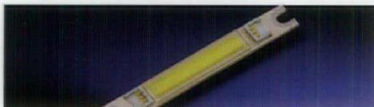
The CL-L100 packs a super luminance flux of 245lm with high efficiency. Space-saving thin package releases flat, well dispersed illumination. Power consumption is 3.5 watts. 50x7mm.
