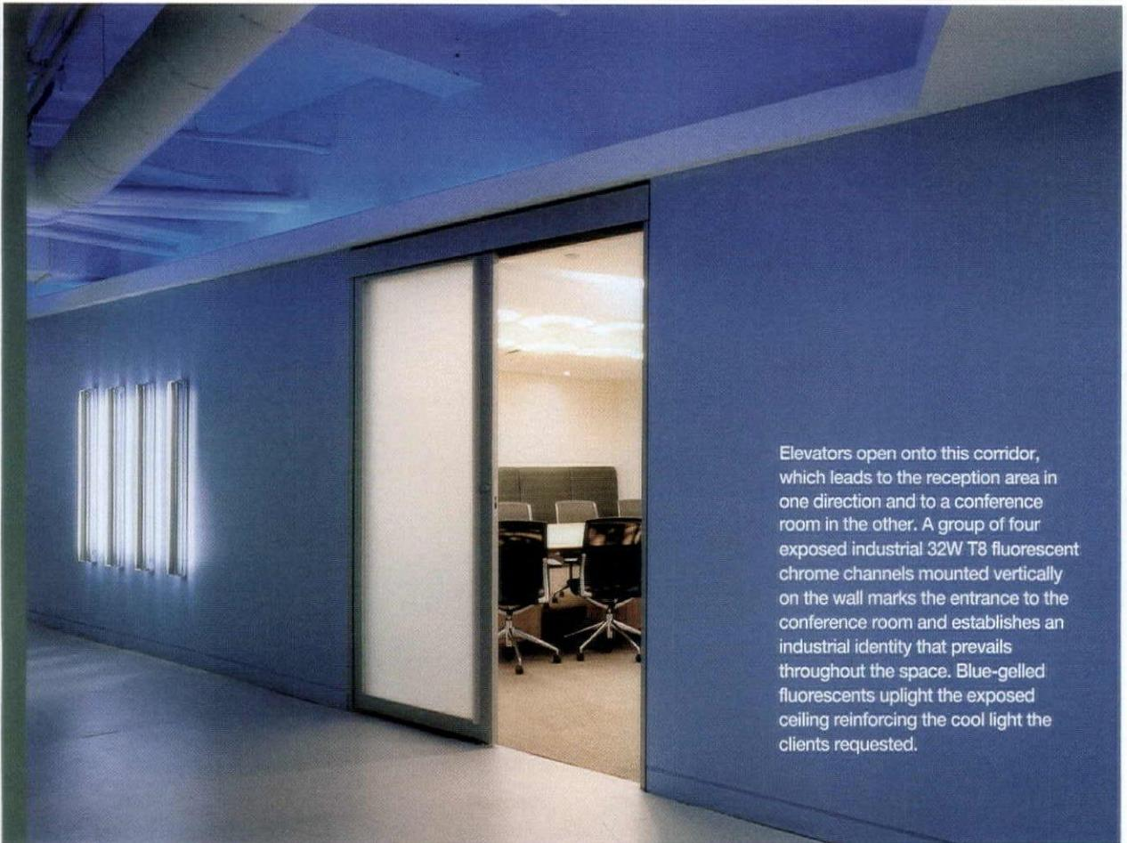
Elevators open onto this corridor, which leads to the reception area in one direction and to a conference room in the other. A group of four exposed industrial 32W T8 fluorescent chrome channels mounted vertically on the wall marks the entrance to the conference room and establishes an industrial identity that prevails throughout the space. Blue-gelled fluorescents uplight the exposed ceiling reinforcing the cool light the clients requested.
