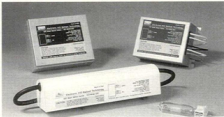
**INnova** has introduced a family of dimmable electronic ballasts for 35-150W metal halide lamps. Features 0.99 power factor, <10% THD, dimming capability and good light output regulation with only a +2% change in light output for a +10% change in line voltage. **Circle No. 228**
