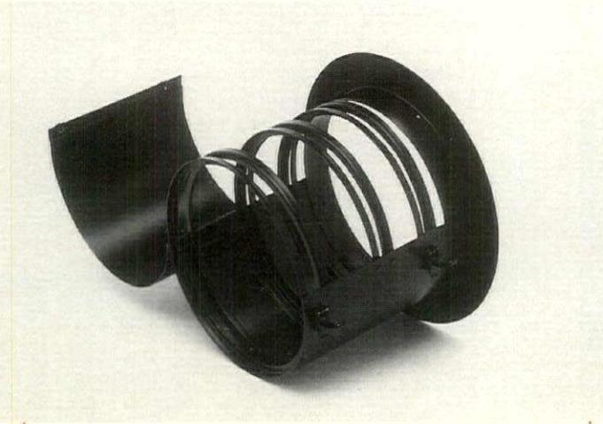
**Phoenix's Snoot Kit** Accessory mounts on the front of fixtures to hold a variety of special effect accessories. The snoot door opens with the release of two stainless steel latches, allowing for installation of accessories. Accessory rings are riveted in place to secure accessories in mounting position. The snoot measures 8 in. in diameter x 8 in. long from fixture doorframe. Housing and rings are copper-free formed aluminum. UL-listed. **Circle No. 248**
