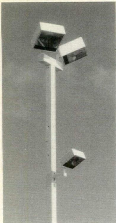
**Ruud Lighting's** Cutoff Floodlight (CF Series) feature die-cast aluminum housings in compact 12-, 16- and 22-in. square sizes with a bronze finish and is protected by Ruud's seven-year warranty. Can be specified with 35W to 1000W HID lamps. Factory-installed options—available, including fusing, two-level operation, photocontrol and quartz standby. UL-listed for wet locations. **Circle No. 196**
