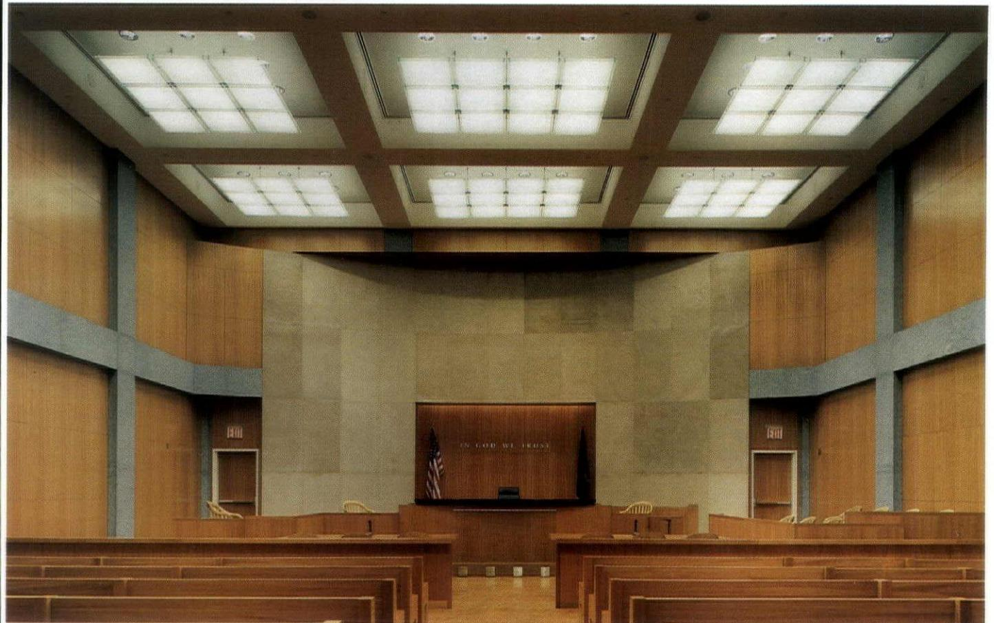
OPPOSITE: LOW-VOLTAGE PAR 16S ILLUMINATE THE COLUMNS, AND FLUORESCENTS IN COVES UPLIGHT THE CORRIDOR CEILING OFF THE FOUR-STORY ATRIUM, WHICH IS FLOODED WITH DAYLIGHT. COMPACT FLUORESCENTS MOUNTED ABOVE ACRYLIC PANELS PROVIDE AMBIENT LIGHT THROUGHOUT THE CEREMONIAL COURTROOM (ABOVE), WHILE PAR 38S HIDDEN IN A CEILING POCKET PROVIDE FOCAL LIGHT ON THE JUDGE'S DESK AND WASH THE BACK WALL.
