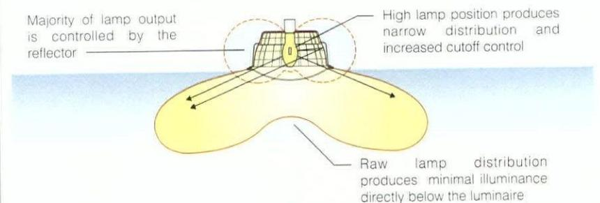
**HIGH VERTICAL LAMP POSITION WITH CONVEX LENS** is well suited for narrow symmetric distributions with sharp cutoff control.
