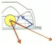
Flat lens surfaces can produce undesirable inter-reflections at shallow incident light angles.
