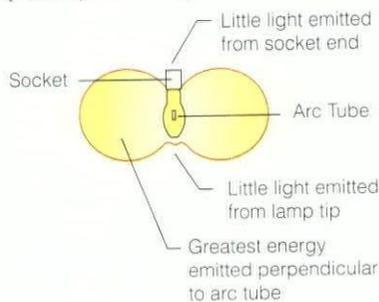
Lamp orientation and the design of reflector components use these characteristics to achieve the greatest end result.
