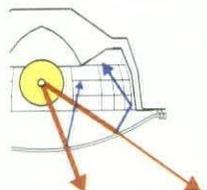
Convex lens reduces inter-reflections, improving luminaire efficiency at high distribution angles.
