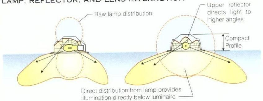
**HORIZONTAL LAMP WITH FLAT LENS** is well suited for asymmetric distributions with very sharp cutoff control.
