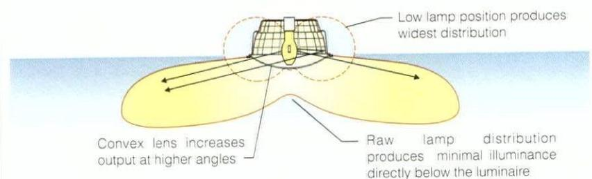
**LOW VERTICAL LAMP POSITION WITH CONVEX LENS** is well suited for wide symmetric distributions.
