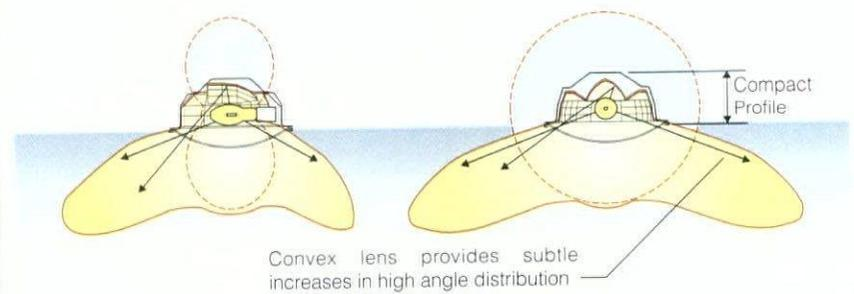
**HORIZONTAL LAMP WITH CONVEX LENS** is well suited for asymmetric distributions with good cutoff control, where increased lens presence is desirable. A subtle improvement in uniformity is also realized.
