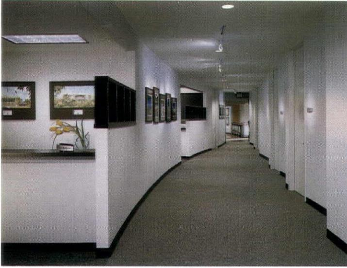
CORRIDORS SHOWCASE PROJECTS DESIGNED BY THE COMPANY AND EXECUTIVES' NAMEPLATES HIGHLIGHTED WITH DIMMABLE RECESSED TRACK MR16 FIXTURES. CIRCULATION PATHS HAVE TRIPLE-TUBE PL FLUORESCENT DOWNLIGHTS—USED FOR THEIR ENERGY EFFICIENCY—WITH EVERY OTHER ONE ON EMERGENCY POWER FOR EGRESS LIGHTING.
