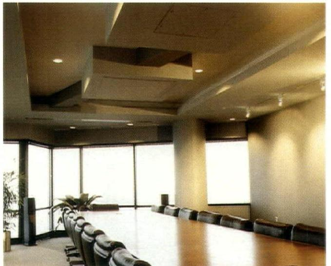
INCANDESCENT DOWNLIGHTS OVER THE TABLE AREA AND ALONG THE PERIMETER ARE SEPARATELY DIMMABLE. CORRIDOR-MATCHING RECESSED TRACK-MOUNTED MR16 FIXTURES HIGHLIGHT VISUAL ELEMENTS DISPLAYED ALONG THE WALL DURING PROJECT PRESENTATIONS TO CLIENTS.
