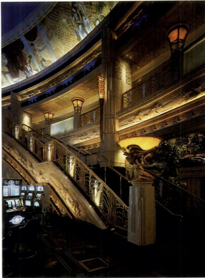
A MIX OF DECORATIVE AND CONCEALED ARCHITECTURAL FIXTURES BRING THE GATEWAY OF ENTERTAINMENT TO LIFE. CONCEALED IN COVES, ROWS OF COLD CATHODE TUBES IN PINK, GOLD AND PALE BLUE ILLUMINATE THE MURAL CIRCLING THE BASE OF THE DOME. THE LAMPS ARE FITTED WITH ROTATING SNAP-ON REFLECTORS FOR BETTER CONTROL AND EFFICIENCY. CUSTOM RADIAL LOUVERS CONSTRICT THE LIGHT OUTPUT FROM ALL COVES AND DIRECT IT TOWARD ENTABLATURES AND MURALS WITHOUT MUTING THE RICH CEILING COLOR.
