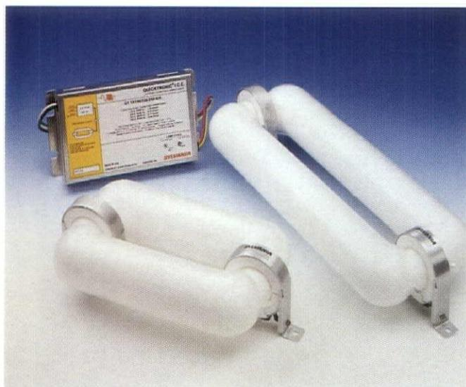
LAMPS SUCH AS OSRAM SYLVANIA'S ICETRON ARE BEING USED IN OUTDOOR APPLICATIONS. THE RECENT RELIGHTING OF NEW YORK CITY'S UNION SQUARE PARK FEATURES THE LAMPS, WHICH USE MAGNETIC-INDUCTION TECHNOLOGY TO GENERATE LIGHT-PRODUCING ELECTRONS INSTEAD OF AN ELECTRODE AT EACH END OF THE FLUORESCENT TUBE—BOOSTING AVERAGE LAMP LIFE TO 100,000 HOURS. THE HPS LAMPS THAT WERE USED TO LIGHT THE PARK FOR THE PAST 30 YEARS OFFERED LIFE RATINGS OF UP TO ONLY 24,000 HOURS. **CIRCLE NO. 43**
