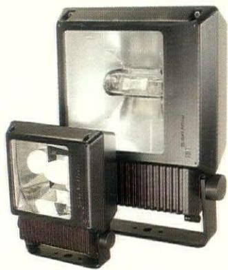
Hydrel/SILL 7800 Series Architectural Floodlights are located at the first setback of the Tower. These fixtures are designed to withstand extremes in temperature, moisture, dirt, mishandling and vandalism. These high-performance, low-glare fixtures in low-profile, compact housings provide eight light distributions and vertical or horizontal mounting. Model 7800 accepts specified HID lamps to 100W, model 7801 to 400W. **Circle No. 67**
