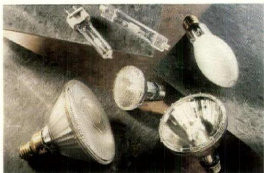
**Philips' MasterColor** lamps were used inside downlights to add direct lighting to the trading floor. MasterColor metal halide lamps feature lamp to lamp consistency over life; high color rendering (82 to 85 CRI for 3000K; 90 to 93 CRI for 4000K); high lamp efficacy (up to 95 LPW) and ALTO lamp technology, which passes the EPA's TCLP test for non-hazardous waste. **Circle No. 43**
