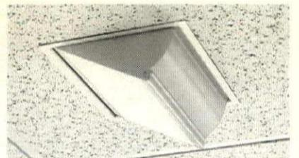
With its shallow recess depth (less than 5"), the **Style 211** fits under ducts at core walls and can be mounted in drywall or tile ceilings. A snap-on, UV filtering, hinged lens allows for relamping without tools. Available with a 32W or 42W Hex Tube lamp for low-energy, long life and great color.
