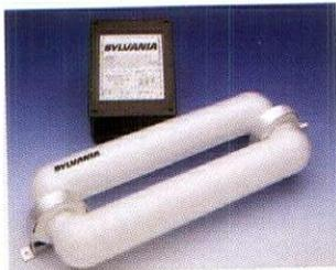
Osram Sylvania's new technology for electrodeless induction lamps uses a magnetic field to generate electron flow (unlike the electrodes used in conventional fluorescent lamps), resulting in an average rated lamp life of 60,000 hours. The new lamp will be available in two system wattages (100W and 150W) and three system lumen packages (7,500, 10,000 and 12,000).
