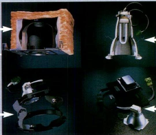
**ADJUSTABLE ACCENT FIXTURES** permit 361° rotation for all optical elements to eliminate common dead spots when aiming lamps, and up to 45° vertical aiming for flexibility. Translating center beam optics provide maximum light output through the aperture over the entire range of lamp tilt. Tool-free locking of the adjustable brackets allows for easy and secure aiming. All MR16 units come with backlight shrouds to prevent light escaping to the platform interior.
