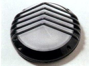
BL-36, 38, 44 and 45 fixtures are an extension of the BL-Series of building-mounted landscape lighting fixtures, which include BL-35, 52 and 55 (shown). Each fixture housing is cast aluminum with a high-impact clear glass or opal polycarbonate lens and extruded aluminum silicon gasket for a water-tight and bug-free seal. Cast aluminum vertical and horizontal lens guards protect fixtures from debris and vandalism. ULC-, ETL-listed for wet location and through wiring. **Circle No. 55**
