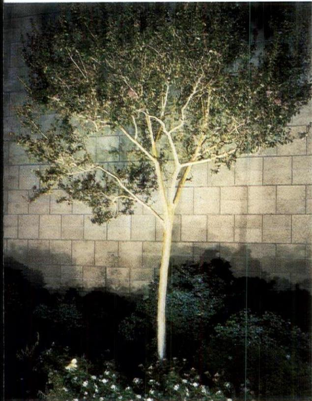
TO LIGHT THIS LANDSCAPE FEATURE OUTSIDE THE PALM SPRINGS CITY HALL, THE DESIGNER SPECIFIED A SINGLE IN-GROUND FIXTURE FROM ALL. THE FIXTURE IS A COMPRESSION-MOLDED COMPOSITE FIXTURE WHICH PROVIDES EXCELLENT RESISTANCE TO CORROSION AND STRESS THAT OCCUR IN ANY LANDSCAPE, PARTICULARLY AROUND TREES AND SHRUBS. **CIRCLE NO. 50**
