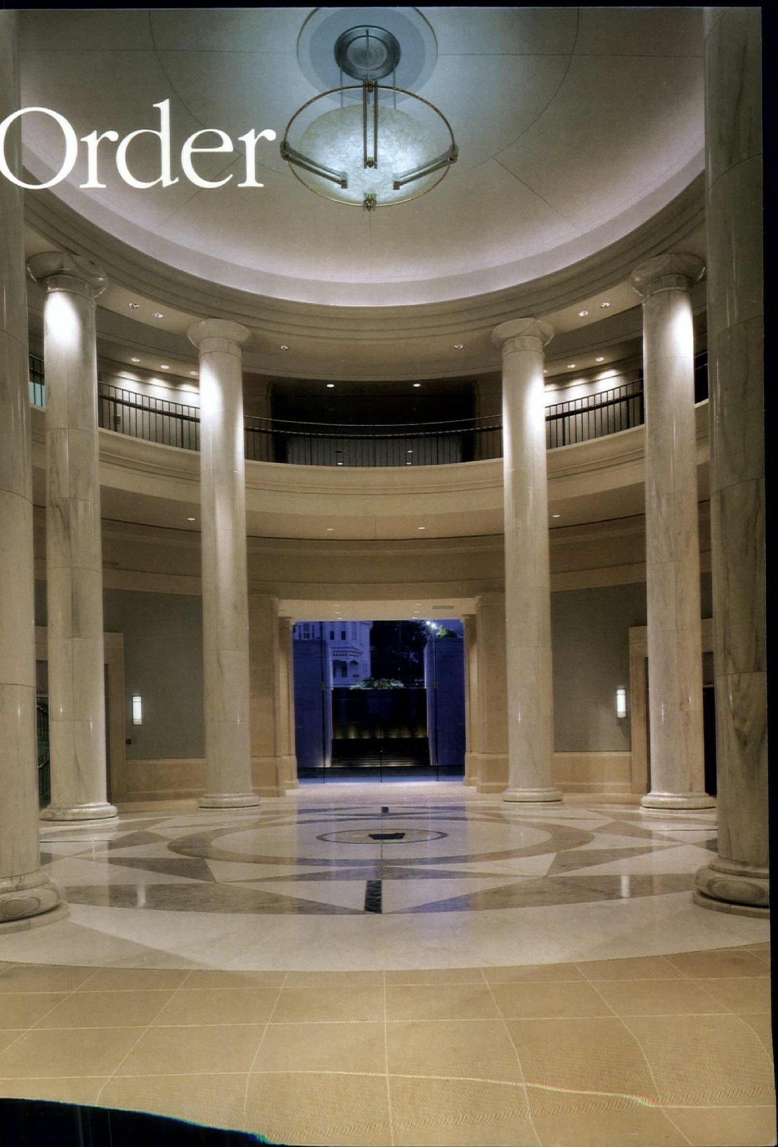
lamps. The fluorescent accentuates the volume of the space and emphasizes the classical architecture. The design team chose indirect lighting for the central space to avoid unwanted reflections and glare on the stone columns and floor, which is polished in the central traffic area.
