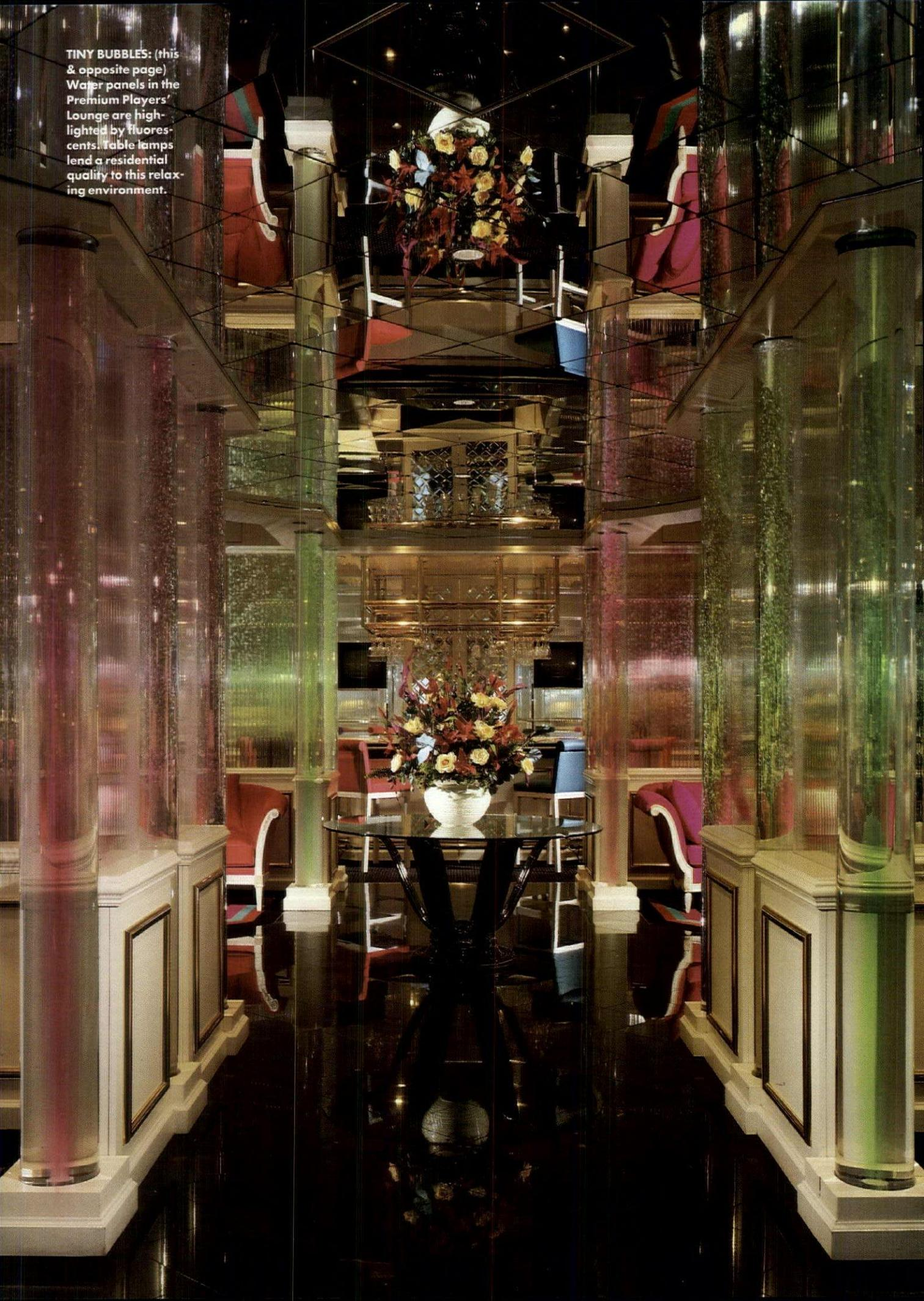
panels and concealed by the millwork trim. Hinged panels allow for maintenance access. Each water-filled circular column has a wet location, 5 1/8-inch-diameter, compact fluorescent upright installed in its base. Holidays and special occasions can be celebrated festively with light by adding colored filters.
