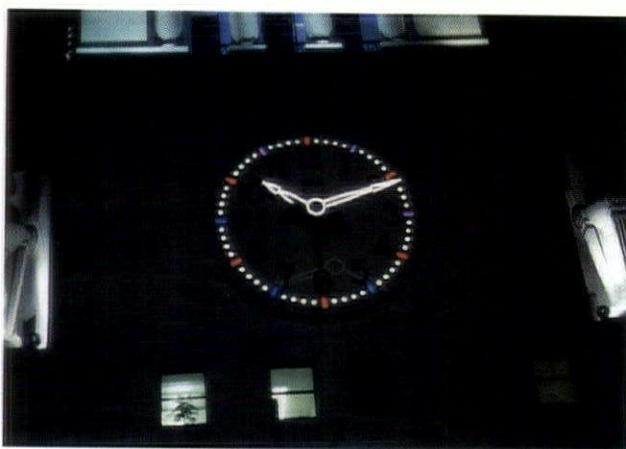
(Right) The old incandescent system used 860 lamps. The new fiberoptic one uses only 44 low-wattage metal halides.
