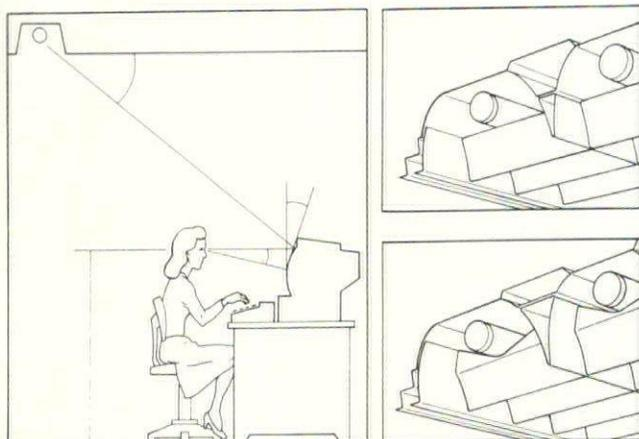
Figure 1: (Left) VDT workstation elevation, (top right) standard parabolic, (bottom right) compound parabolic.
