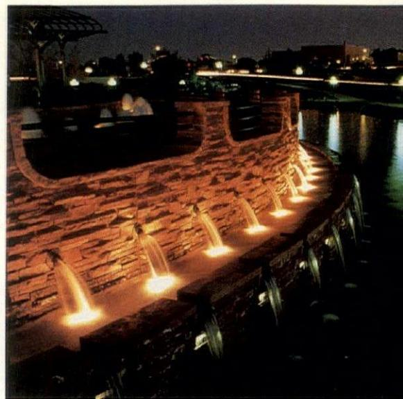
and two levels of cascading waterfalls that return the water to Little Dry Creek. The spouts of water empty into the mid-level, and the falls and masonry are highlighted from below by 250-watt incandescent PAR lamps. The lower waterfalls are lit from behind by 13-watt PL fluorescent lamps.
