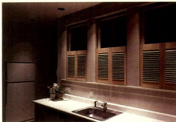
**TASK MINUS AMBIENT EQUALS GLOOM:** Task lighting from recessed incandescent luminaires without ambient lighting creates a gloomy space.
