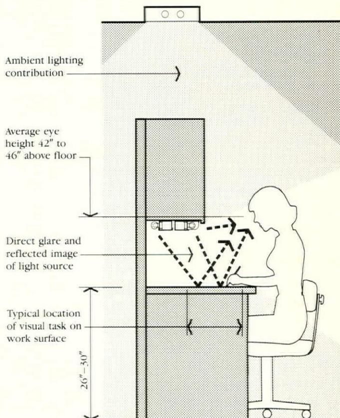
*Unshielded under-cabinet task lighting can cause direct glare from the luminaire and reflected glare from an image of the light source on the visual task.*
