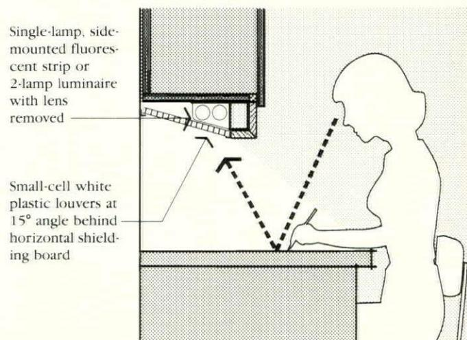
*Small-cell louvers installed at an angle underneath the lamps shield the reflected lamp images, which reduces the lighting level but substantially increases task visibility.*
