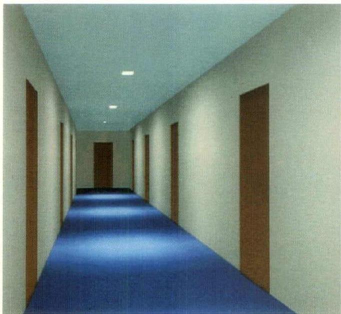
*Lumen-Micro Targa-16 results produce screen displays of simulated room lighting — in this example, two images*
