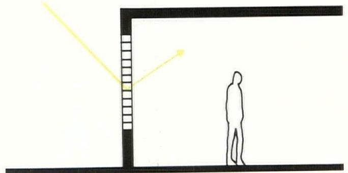
*Light-directing glass blocks have built-in prisms that can be used to refract light toward the ceiling.*
