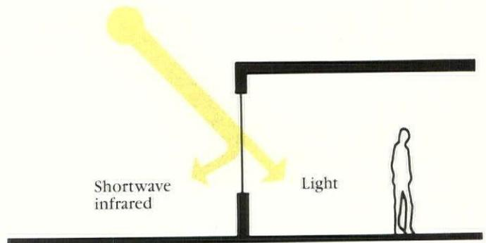
*The ideal selectively transmitting glazing would reflect all of the sun's infrared radiation and would allow the visible light to pass through.*
