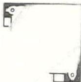
Elliptipar's concealed fluorescent reflector outperforms all alternatives for cove and perimeter "slots." Even illumination, no harsh socket shadows, and small cross section in lengths of 2, 3, 4, 5, 6, 8 and 10 foot (nominal). Economical to purchase & operate.
