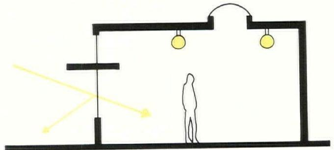
*Tinted or reflective window glazing will reduce glare only if the space is lighted by other sources, such as electric lights or skylights.*
