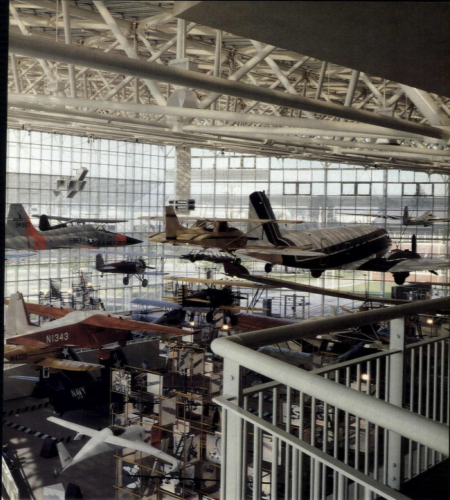
The triple-glazed reflective roof caused the highest heating and the lowest cooling loads; the Heat Mirror caused the opposite effect and admitted only a small amount of additional daylight. The triple-glazed reflective glass was eventually selected for use on the roof because the glazing would be installed in
