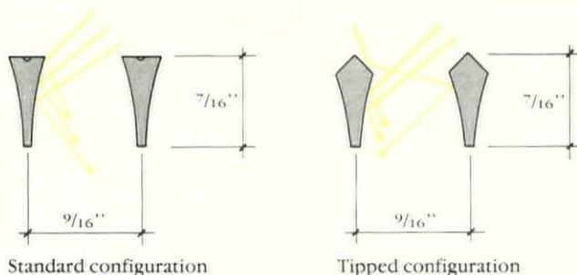
*The diagram on the left shows how light rays bounce off the surface of the parabolic curve. The height of the louver determines the cutoff angle. Specularity affects the direction in which the rays bounce. Adding a dome at the top, as shown on the right, can force more light downward.*
