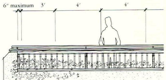
*Elevation of lighted guardrail planter demonstrates the use of combined 3-foot and 4-foot fluorescent light strips to achieve overall lengths in 1-foot multiples. To minimize dark areas between lamps, use strips without end caps and install lamps back to back.*
