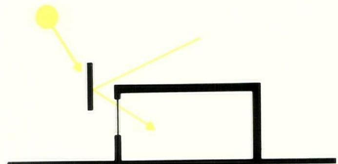
*A vertical panel can block direct sunlight while reflecting diffuse skylight.*
