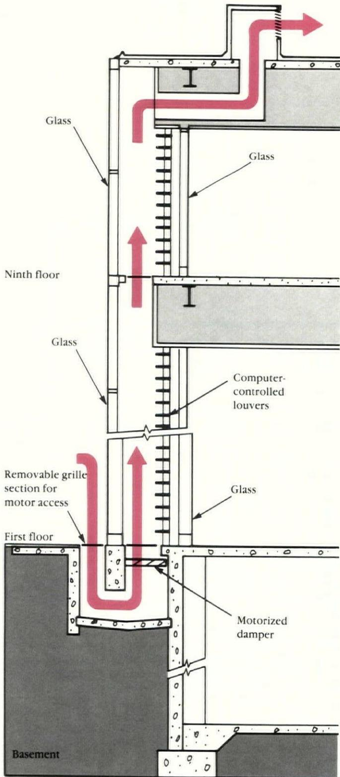
*The Hooker Office Building, Niagara Falls, New York, uses computer-controlled louvers to regulate the light and heat entering the building.*
