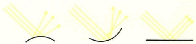
*Both concave and convex specular reflectors can be used to distribute daylight over a wide area of the ceiling.*
