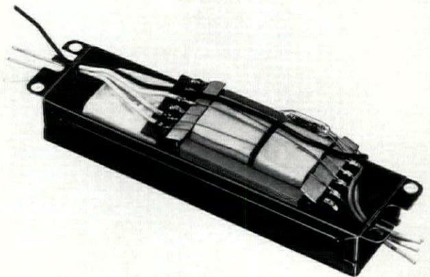
*Demonstration model of a core-and-coil ballast shows inner components. A small, glass-enclosed thermal protective device rests atop the core-and-coil assembly. The capacitor at left, fastened to the assembly beneath lead wires, provides power factor correction. In a usable ballast, potting compound surrounds the components, completely filling the case.*
