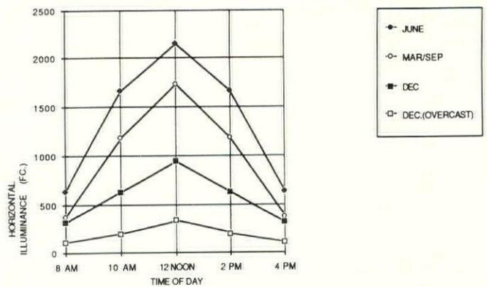
HORIZONTAL ILLUMINANCE AT THE CENTER OF THE ATRIUM FLOOR AT 4 FEET HEIGHT AS A FUNCTION OF TIME OF DAY AND MONTH GREENWICH-CONNECTICUT
