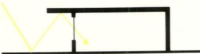
*Large horizontal overhangs block too much light unless both the ground and the underside of the overhang have high reflectance values.*
