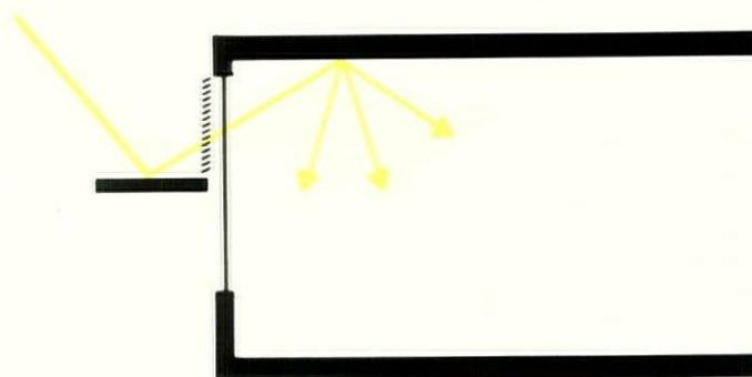
Light shelves act as overhangs for the view windows beneath; louvers can be used to avoid glare caused by the glazing above the light shelf.
