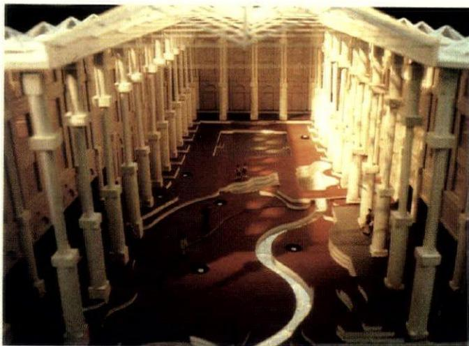
*1/4-inch scale model of the atrium used for daylighting studies. Photometers are visible on model atrium floor.*
