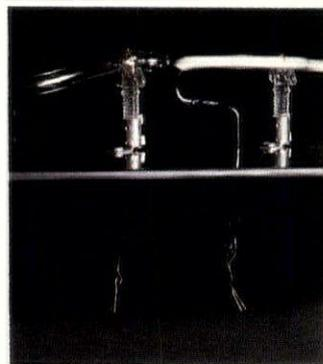
*Detail of an unfinished neon sculpture shows clear and coated glass on a plastic mounting board. Note black-out paint, glass tube supports in metal bases, copper tie wire, and electrodes passing through holes in surface.*
