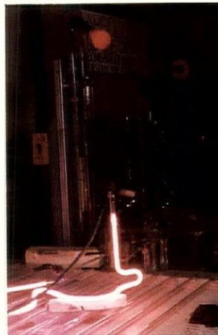
*Bombarding the empty lamp with a 15,000-volt charge. A thin glass tube connects the lamp to the gas manifold.*
