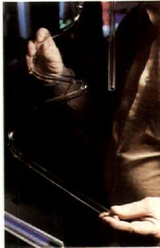
*Lowering the tube over a ribbon burner. Red marks show which sections to heat for a gentle curve.*
