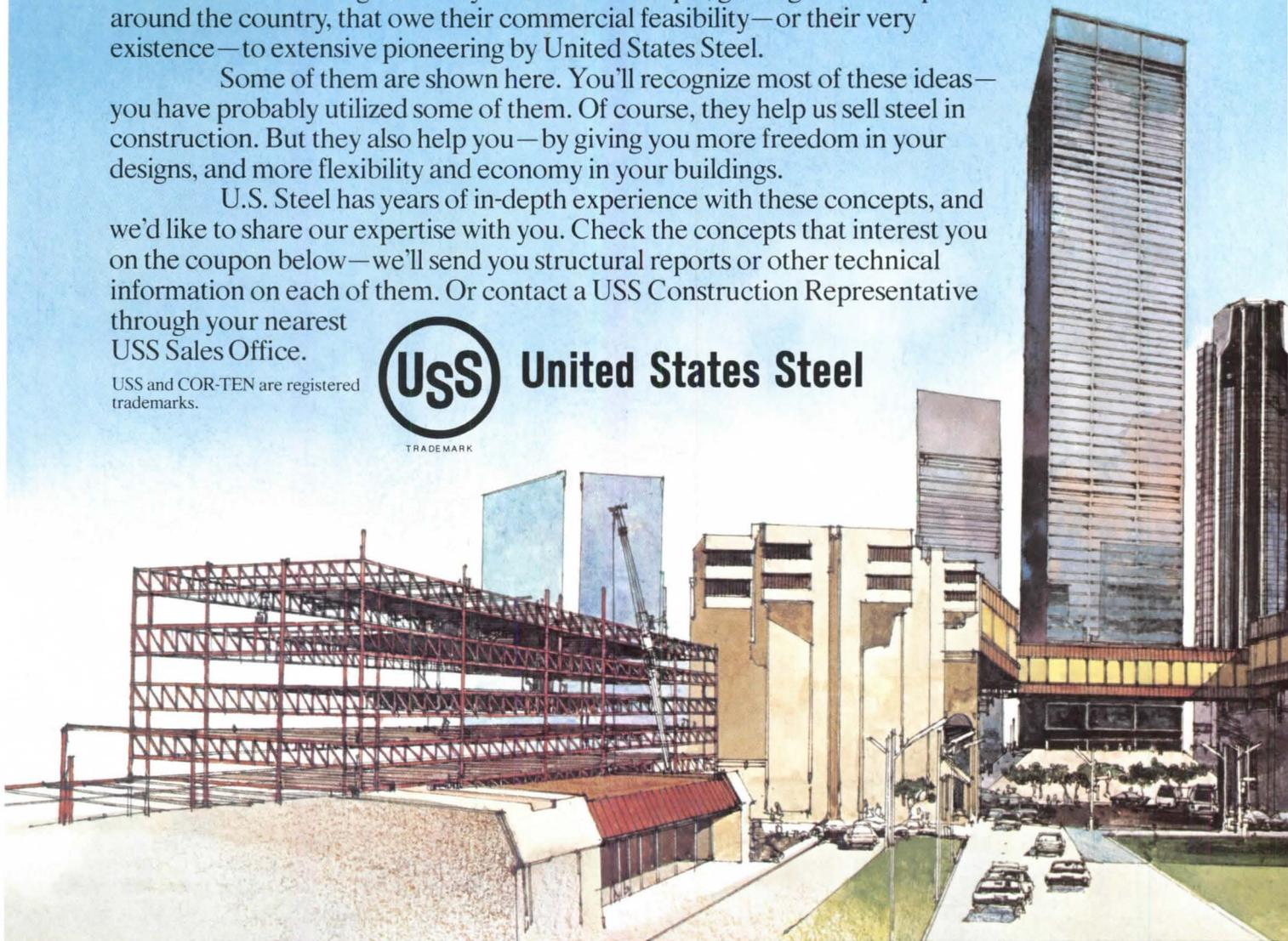
**Interstitial Space Design.** A series of structural steel 'sandwiches' or full height service levels between working floors—in which mechanical, electrical communication lines and distribution and collection systems can be housed and maintained. Over the past 6 years, 35 hospitals have been designed with it.
