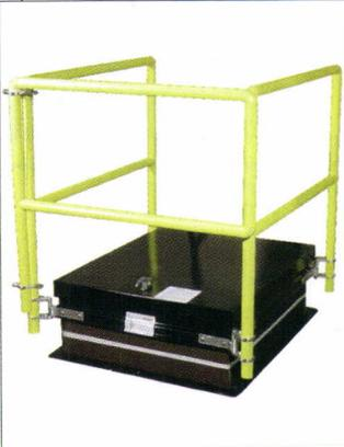
Bilco's Bil-Guard™ hatch railing system provides a permanent means of fall protection for hatch openings. Tested and proven to meet and exceed OSHA fall protection regulations (29 CFR 1910.23), the Bil-Guard installs easily with basic tools and features corrosion resistant construction. For more information, visit [www.bilco.com](http://www.bilco.com) or call (203) 934-6363. **Circle 103**
