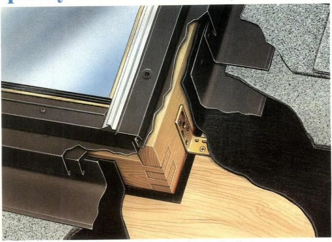
Precision engineered pre-fabricated flashings eliminate the need for caulking.
