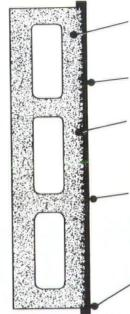
Lightweight structural concrete masonry units
