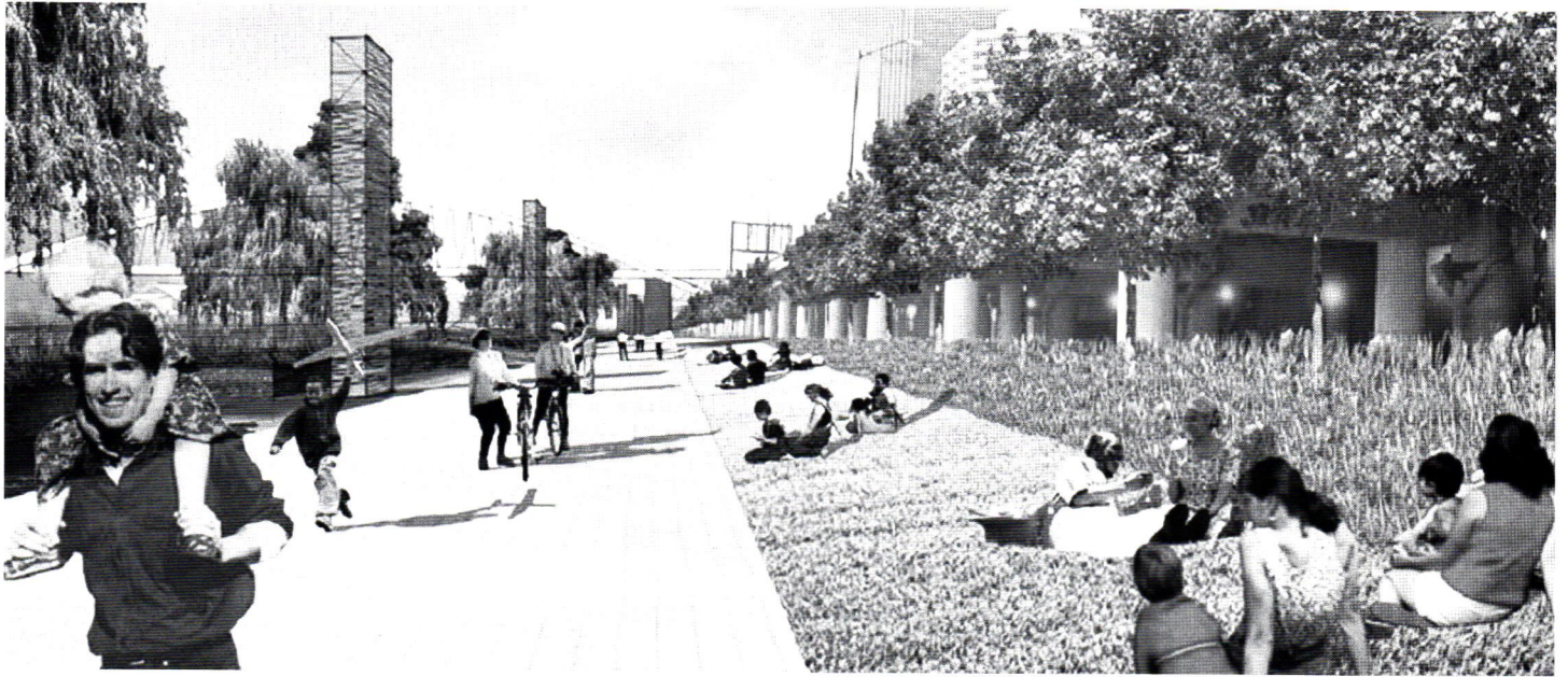
The rendering depicts a portion of the preliminary design for "Mon Wharf Landing" developed by Hargreaves Associates. It shows the two main components of this plan which are: 1) A trail connection and landscaped edge on the land side (both of which would be designed to withstand flooding) and 2) A barge-based landscape on the water side, part of which could be designed to help collect and treat highway runoff from the roadway above the Wharf. These barges could also be programmed to provide additional park and activity space, recreational boating tie-ups and many other uses. Riverlife recently received a transportation enhancements grant for funding to begin Phase I construction of the land-side landscaped berm and trail that will ultimately connect the Eliza Furnace Trail with Point State Park.
