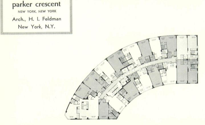
The problem was the design of an apartment building on an irregular plot. The rear of the plot is a continuous curve formed by the approach to the Midtown Tunnel. Few buildings have been built fronting on a similar right of way, and the laws determining the status of rights of way are not clearly defined.
