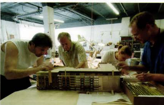
A compilation of building models from around the world greets visitors to Feyereisen Studios (opposite). For Bob Feyereisen, Assoc. AIA, the model-making process includes preparing drawings that ensure the accuracy of the computer-guided router (top), hand assembly (above middle), and preparing a jig for the model installation (lower middle). Mitch Getta, Ron Hansen, Karen Tyvoll and Feyereisen pitch in on assembly (above).
