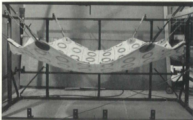
Synclastic structural membrane subjected to surface load.
