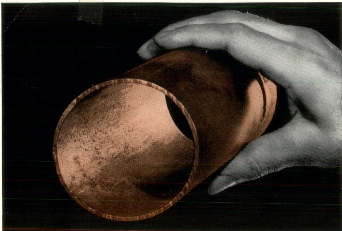
Unretouched photo of 3" dia. copper tube removed after 13 years' service in a soil line.
