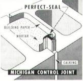
Williams "Perfect-Seal" (Pat. Pend.) is a specially designed seal for use in Michigan Control Joints . . . it provides continuous six-point pressure-contact sealing which keeps moisture out of joints and prevents air passage. The T-Section is a high-grade rubber compound; the cross-sealing member at the base of the "T" is a strip of readily compressible, non-absorbent, expanded closed-cell Neoprene Rubber—it provides an effective pressure-contact seal directly behind the calking.
