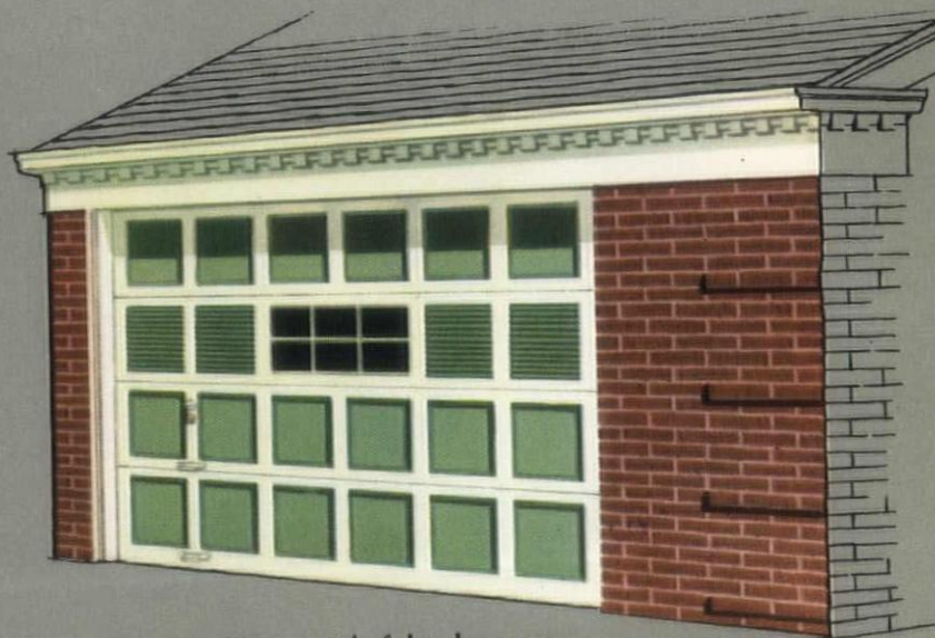
Single-Car Muntin Door with false louvers in harmonizing colors in side panels.
