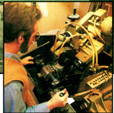
Knife grinder. Using a template a workman grinds a series of knives which enables the Molder to duplicate exact profiles of a 100 year old custom wood molding from a building undergoing restoration.
