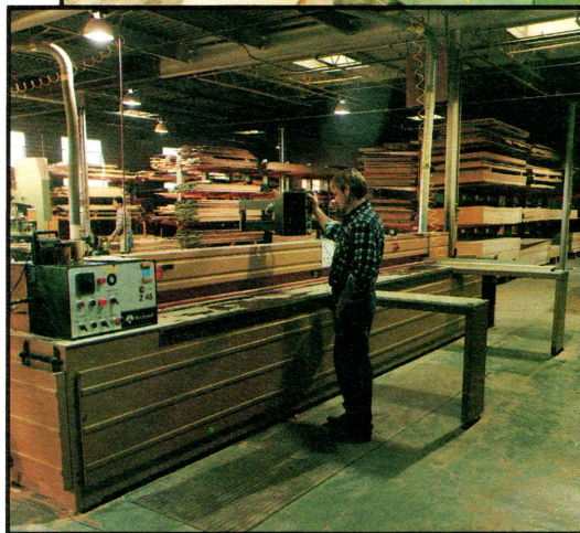
Electronically programmed panel saw with the ability of doing repetitive crosscutting with less than .01 variation.
