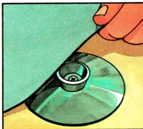
1 Roll membrane over knobbed base plate.
