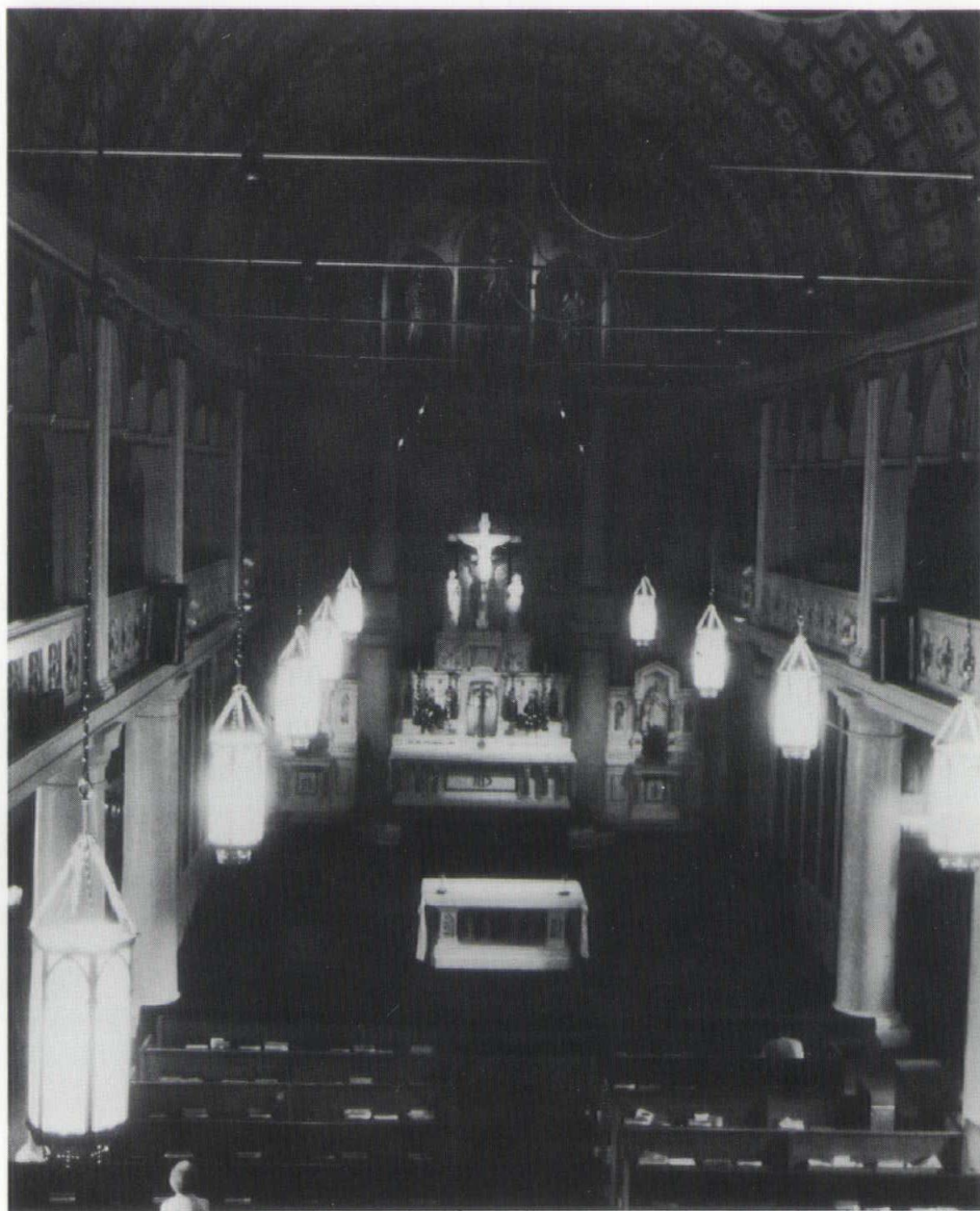
The inherent elliptical pattern of the 25-watt PAR 36 NSP (narrow spot) 12-volt lamp was used to illuminate individual statues adjacent to the crucifix. Approximately 75 foot-candles was achieved from a distance of 20 feet.
