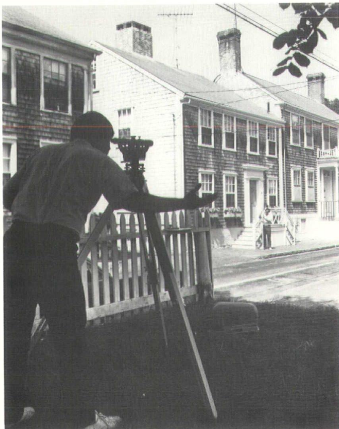
India Street, one of Nantucket's historic passages, is measured with transit and level rod by Ben Walbert and Richard Crisson.
