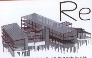
Columns utilizing reclaimed pipe (in red). Revit model by KL&A. Project Structural Engineer and Steel Detailer: KL&A, Inc.
