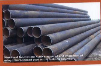
Reclaimed steel gas pipe re-used in the structural frame of the NREL Research Support Facility, the largest Zero Energy Building in North America.
