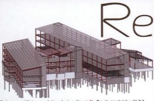
Columns utilizing reclaimed pipe (in red). Revit model by KL&A. Project Structural Engineer and Steel Detailer: KL&A, Inc.
