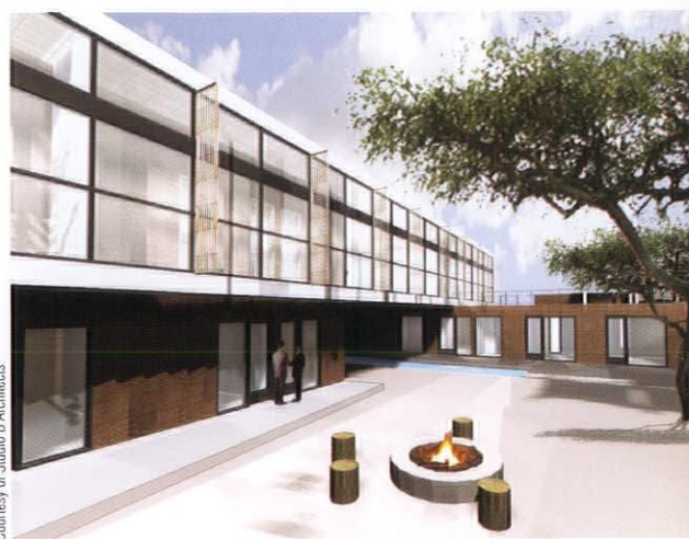
Above and below: Indigenous materials such as mud bricks will be first choice for the unbuilt home. On top of the roof is a system for collecting rainwater as well as PV screens to trap solar energy. Sticks from the area will be used as lattice work, in the ceilings and in operable screens.
