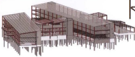
Columns utilizing reclaimed pipe (in red). Revit model by KL&A. Project Structural Engineer & Steel Detailer: KL&A, Inc.
