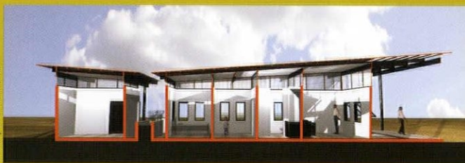
Above High, screened windows let light in and hot air out in Scott Lindenau's design for a school and orphanage in Zambia.
