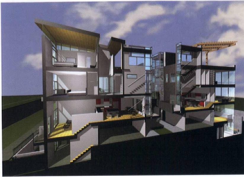
Left: As with many of Colistra's designs, the 11-unit Trellis townhomes are very much about letting in as much Denver light as possible. The facade will be constructed of glass-fiber-reinforced-concrete panels that will contain a computer-generated pattern.
