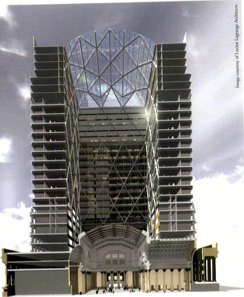
The proposed vertical expansion of Union Station, seen here in section, would preserve the original barrel-vaulted roof as the ‘floor’ of a central atrium whose new 21st century roof then mimics that shape.
