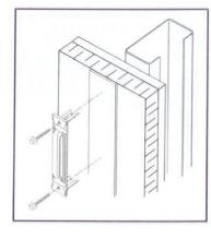
CAPABLE OF WITHSTANDING A 100# LOAD IN BOTH TENSION AND COMPRESSION WITHOUT DEFORMING OR DEVELOPING PLAY IN EXCESS OF 0.05"
