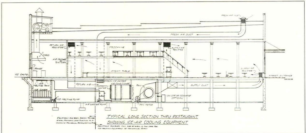
Two-outlet system for restaurants. One supply grille, with the aid of an exhaust grille over the steam table, serves the ground floor, and the other supply grille cools the mezzanine, and also aids in the cooling of the first floor
