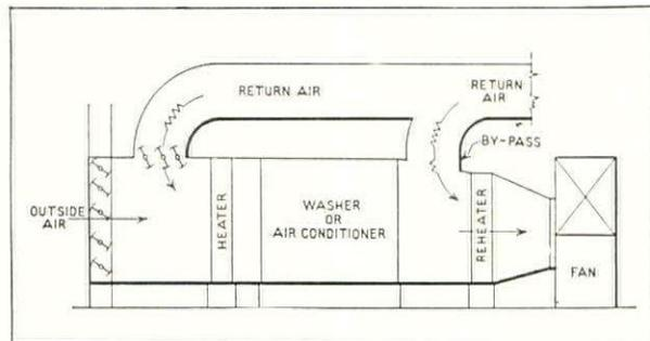
Diagrams of the two methods of air recirculation. At the left is the simple type, in which all the returned air is recirculated; and at the right is the patented method, in which part of the recirculated air is by-passed and the rest reconditioned
