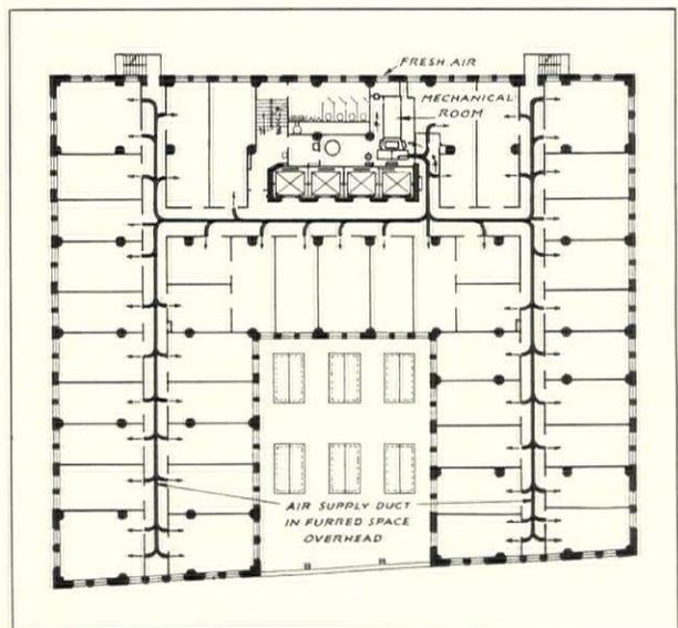
Floor plan and duct layout for the Milan Building, San Antonio, Texas. Air is supplied through grilles in the permanent corridor partitions and withdrawn through grilles in the doors. The corridors are return air ducts
