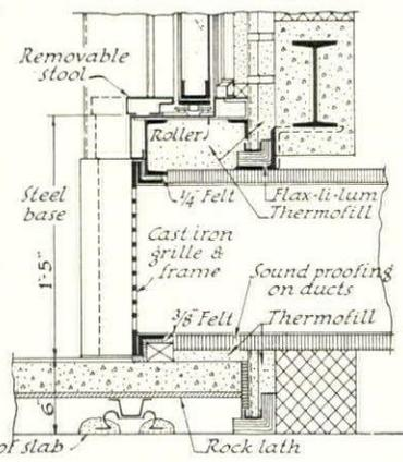
SECTION THRU METAL PILASTERS
