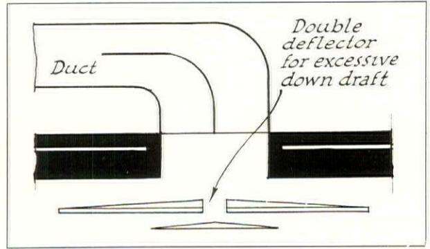
Three different types of outlets, all of which are good practice. At the left is a photograph of one method of architectural treatment for the high pressure nozzle type of distribution. Directly above is a new development in the drop panel type, used when the area to be cooled is large and the air supply is being released at high velocity. At the bottom is a new method of distribution employed with false ceiling construction when it is inadvisable to install outlets in the ceiling itself
