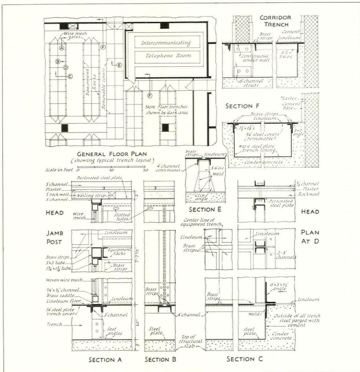
Details of the equipment rack and floor construction of the sixth floor, which is devoted entirely to operating offices, laboratories, and broadcasting equipment. The large amount of conduit that had to be provided for necessitated the use of trenches, 13 in. deep, covered by removable plates so that they could be reached for repair without difficulty. The details at the left, showing the equipment racks, represent a new method of rack construction
